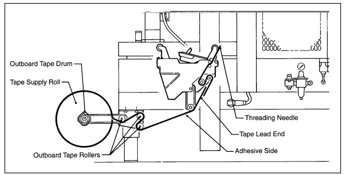
Figure 3-5 – Tape Threading With Alternate Outboard Tape Drum
